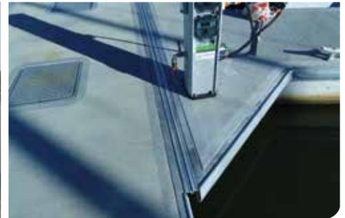
Super Elite™ pontoons are a 5-sided, all-concrete, single monolithic design with the EPS core enclosed in HDPE. Single units range in widths from 1 up to 6 metres, and can be manufactured in any length up to 18 meters per unit. Any number of units can be connected for marina use by utilisation of our custom aluminium waler and hinge assembly. Large 316 grade stainless steel bolts and rubber joints can also be used to form continuous walkways of any desired length when used for wave attenuation
